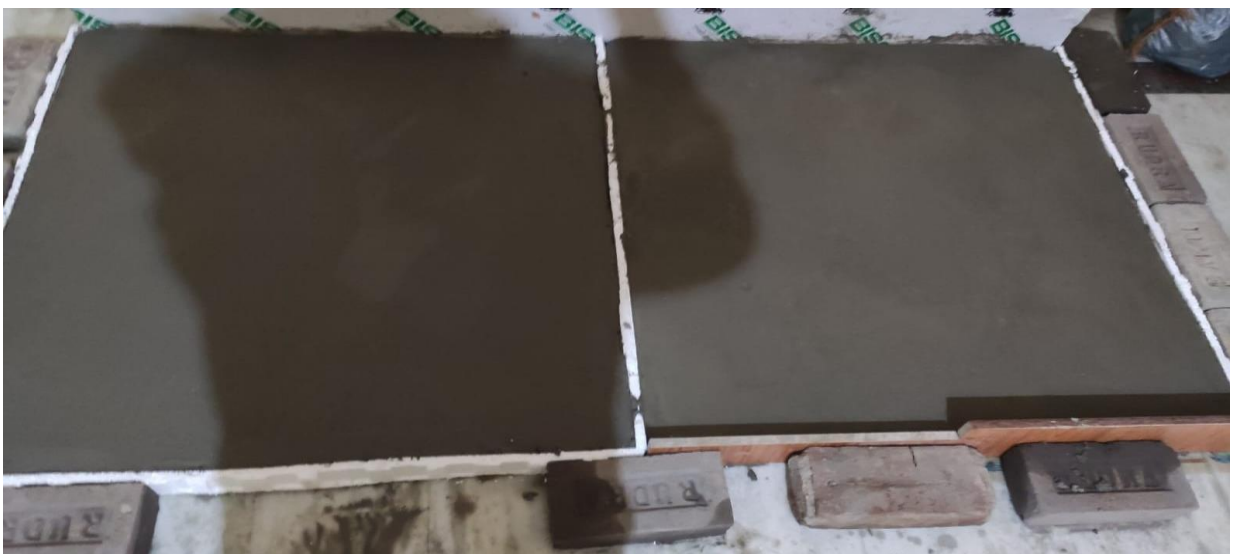
Figure 27. Fabrication of two concrete slab
