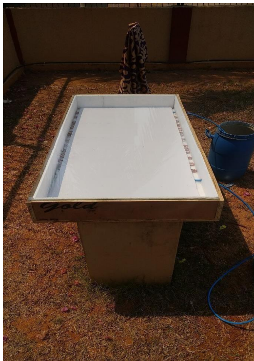
Figure 4: Experimental setup of radiative cooling potential device.
