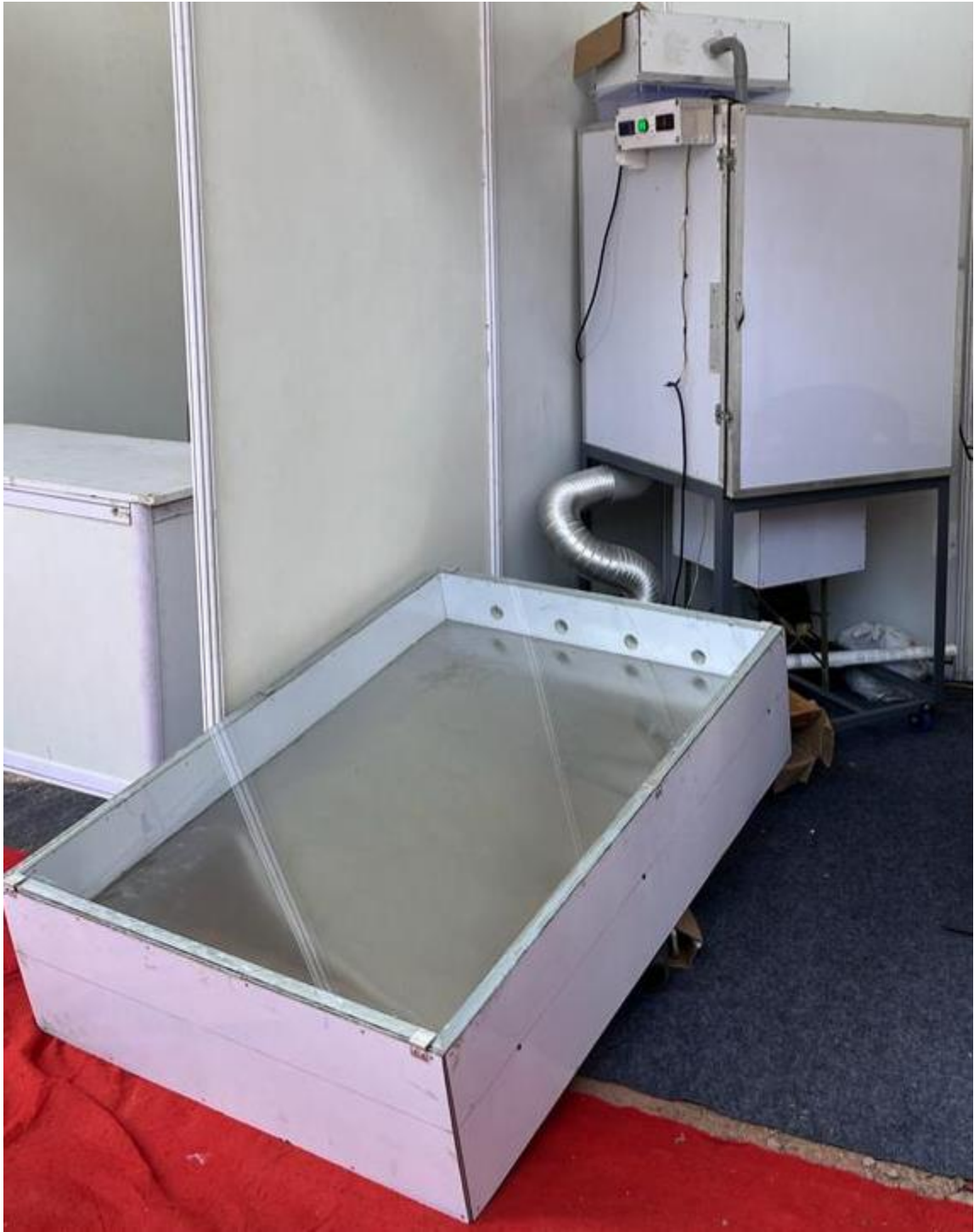
Figure 20 SOLAR ASSISTED HEAT PUMP DRYER
