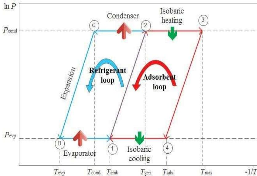
**Figure 2.2: Single bed Adsorption cooling cycle on Clapeyron's diagram.**
