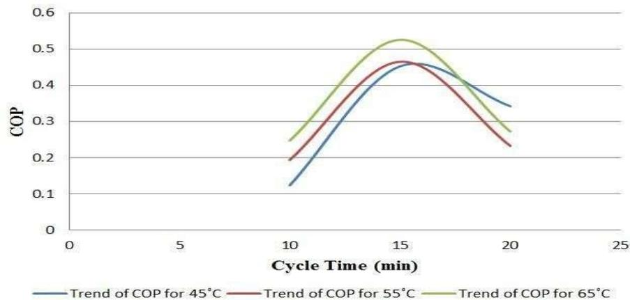
**Figure 5.1: Trend of COP at different Cycle time for a Constant mass flow rate of the hot and cold source**
