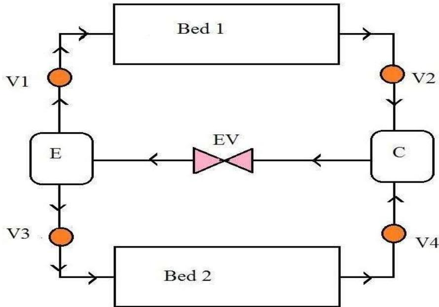
**Figure 2.3: Double Adsorption refrigeration system**
