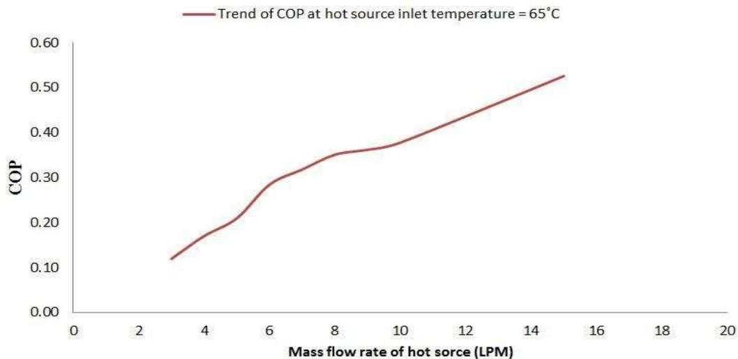
**Figure 5.3: Trend of COP for a different mass flow rate of the hot and cold source at 65°C of hot source inlet temperature**
