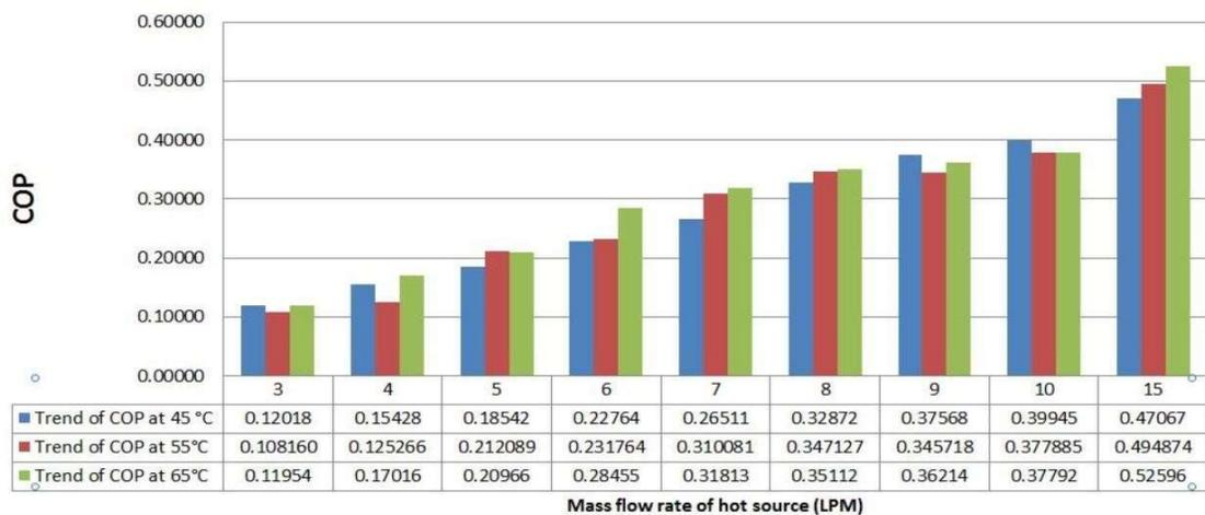
**Figure 5.5: Comparison of COP values in the range of operating conditions for varying mass flow rate of hot source at constant Cycle time**
