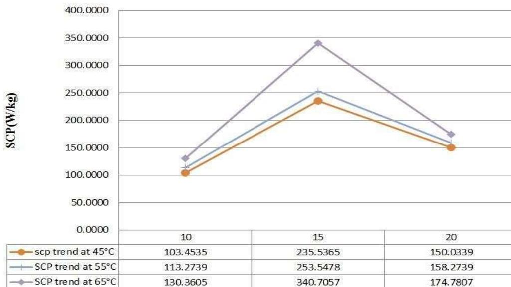
**Figure 5.11: Trend of SCPs in the range of operating conditions against Cycle time at constant mass flow rate of hot and cold source**
