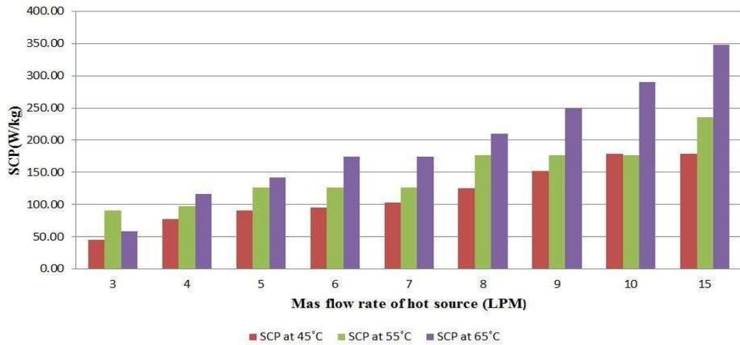
**Figure 5.10:- Comparison of SCP values in the range of operating conditions for varying the mass flow rate of the hot source.**
