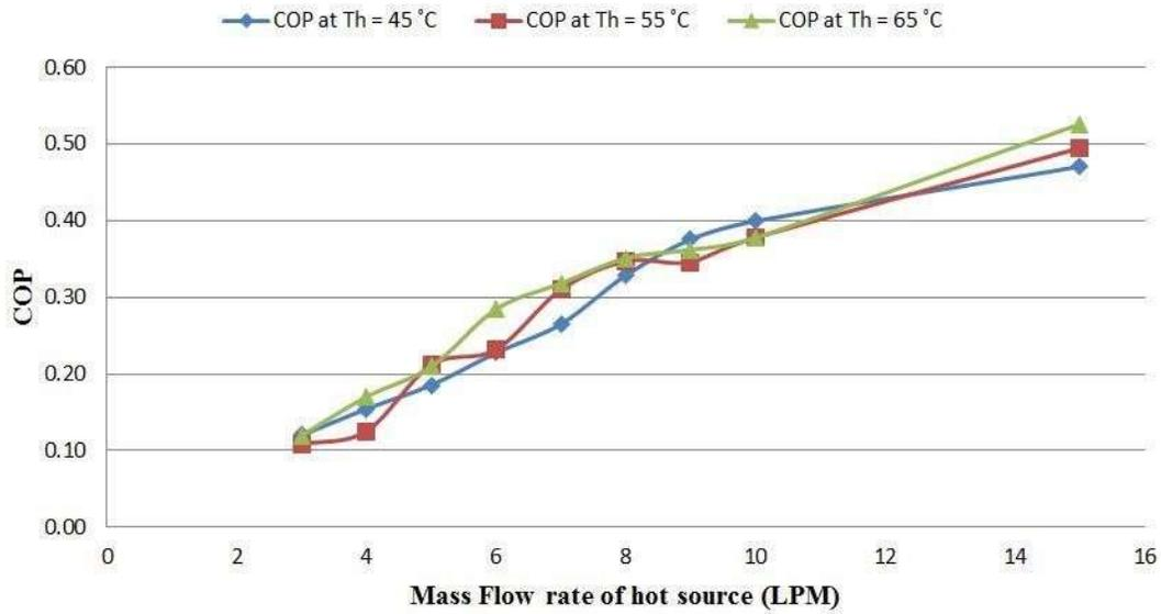
**Figure 5: Different COP Trends obtained at different inlet temperatures of hot source against mass flow rate of hot source at constant Cycle time.**
