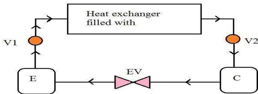
**Figure 2.1:-Single bed adsorption refrigeration cycle[1]**
