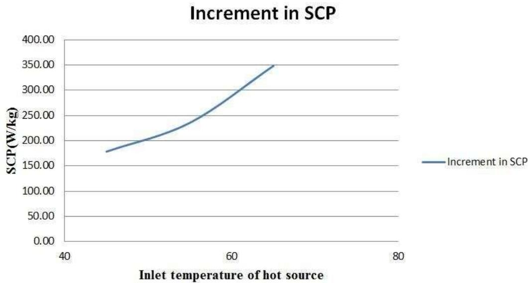
**Figure 5.13: Effect of the inlet temperature of the hot source on Specific Cooling Power (SCP)**
