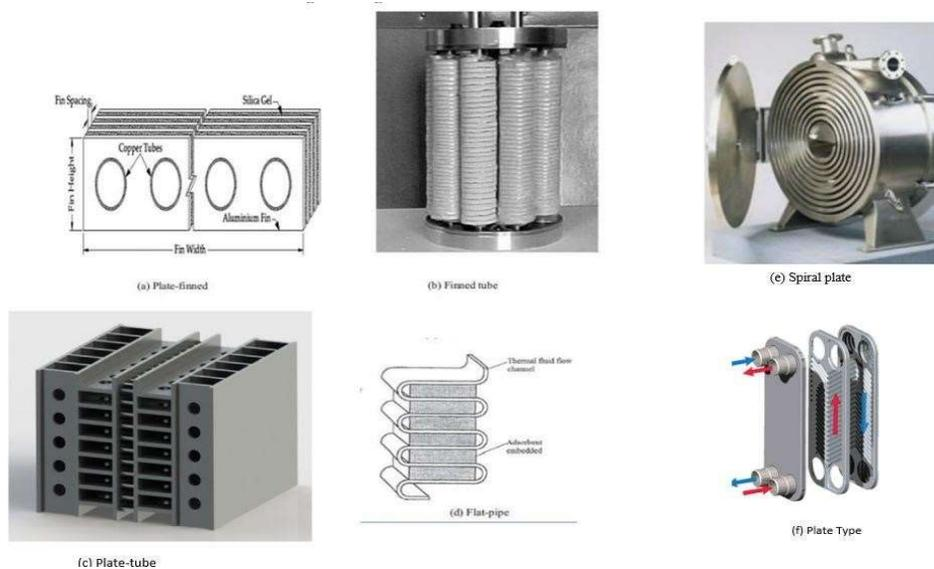
**Figure 3.2: Different types of Adsorber bed heat exchanger configurations**
