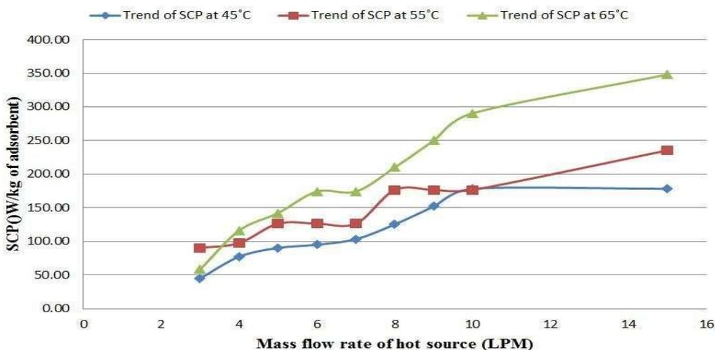
**Figure 5.9:- Trend of SCPs against varying Mass flow rate of the hot source in the range of operating conditions**
