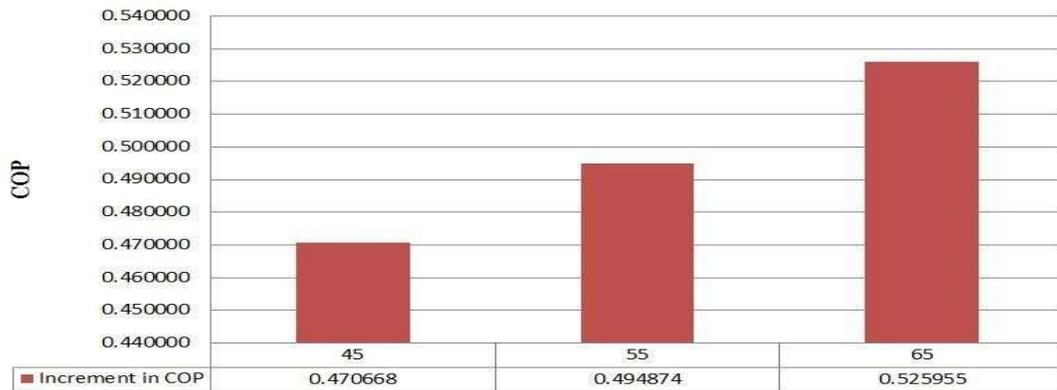
**Figure 5.7: Increment in COP at different temperature of hot source**
