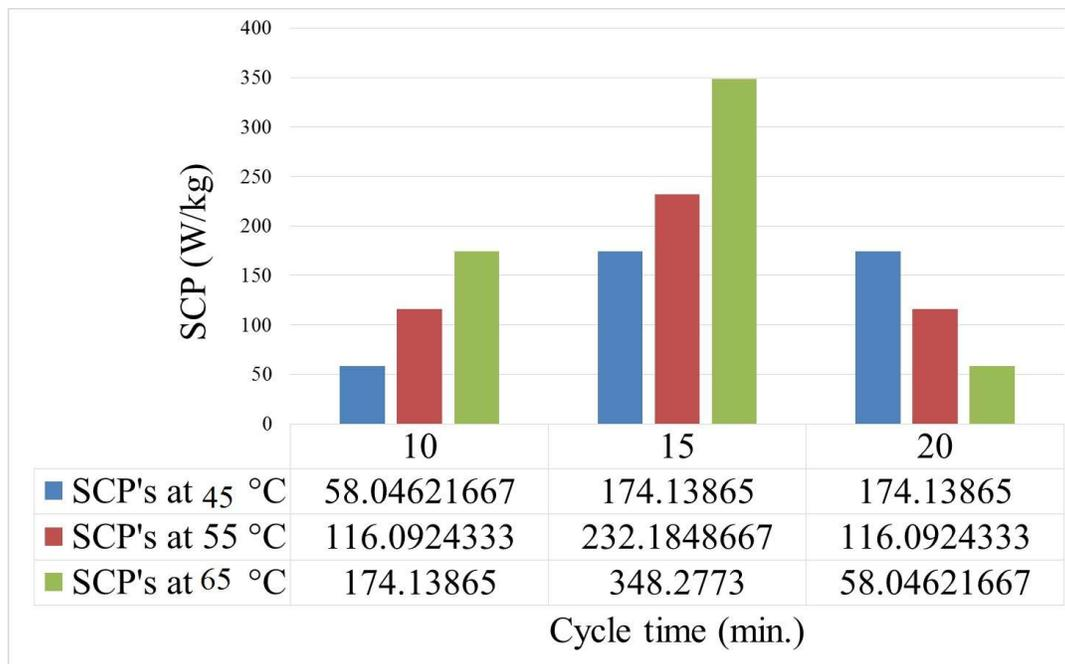
**Figure 5.12 :-Comparison of SCPs in the range of operating conditions against Cycle time at a constant mass flow rate of the hot source**
