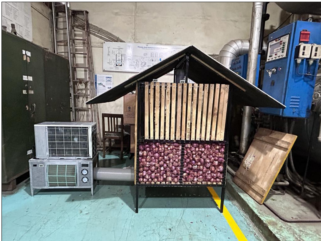
Fig 17: Actual Experimental Setup filled with onions
