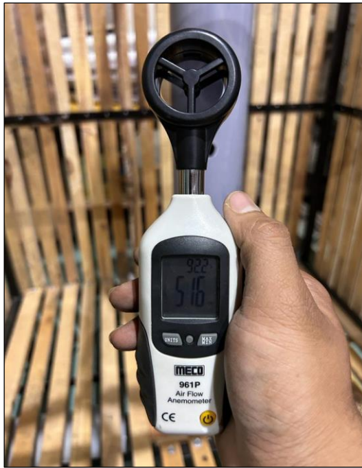
Fig 26: a) Duct Opening Flow without Onions
